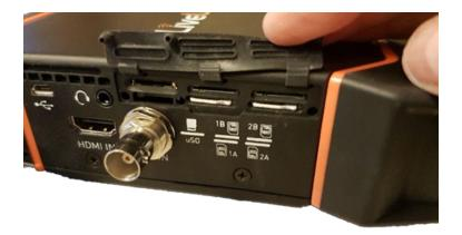
The slots are numbered from 1 and 2, left to right. The bottom row is for SIMs A. The top row is for SIMs B (also indicated on unit). The internal modems use a micro-sized SIM card.
