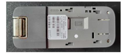
3. The USB modems use a nano-sized SIM card. Align the replacement SIM card as shown below and push into the modem and make sure it clicks into position. If the SIM card does not lock into position, please check SIM orientation and try again.
