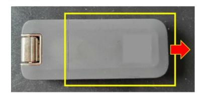
2. If the modem already contains a SIM, eject the existing SIM card by pressing the SIM card into the modem slot. The SIM card should pop out.
