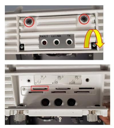
The slots are numbered from 1,3,5 right to left on the top row. The bottom row is labeled 2,4,6 right to left. The internal modems use a full size standard-sized SIM card
