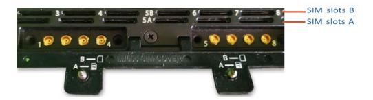
3. Insert the SIM cards labeled 1A -8A on the SIM card sheet in slots 1A - 8A on the unit.
